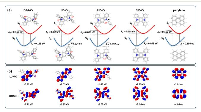
Fig. 2 (a) Optimized  $S_0$  and  $S_1$  geometries and reorganization energy ( $\lambda_{\parallel}$  and  $\lambda_{\parallel}$  correspond to the  $S_1 \to S_0$  and  $S_0 \to S_1$  transition process) of DPA-Cz, ID-Cz, 2ID-Cz, 3ID-Cz, and perylene. All of the optimized geometries were calclulated using the B3LYP functional at the 6-31G (d,p) basis level. (b) Frontier molecular orbitals (HOMOs and LUMOs) and energy levels of DPA-Cz, ID-Cz, 2ID-Cz, 3ID-Cz, and perylene.
