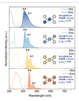
Fig. 1 UV/Vis absorption (dotted lines) and emission spectra (solid lines) of four IDCz model compounds in toluene solution (1  $\times$  10<sup>-5</sup> M).  $I_{0-1}/I_{0-0}$  is the intensity ratio of the vibrational 0-1 peak to the central 0-0 peak.
