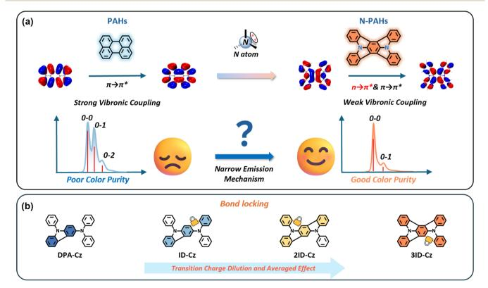
Scheme 1 (a) Schematic diagram of emission spectrum narrowing caused by  $n \to \pi^*$  electron transition (from polycyclic aromatic hydrocarbons (PAHs) to nitrogen atom-containing polycyclic aromatic hydrocarbons (N-PAHs)). (b) Molecular design of four IDCz model compounds: the electron density dilution on benzene rings.
