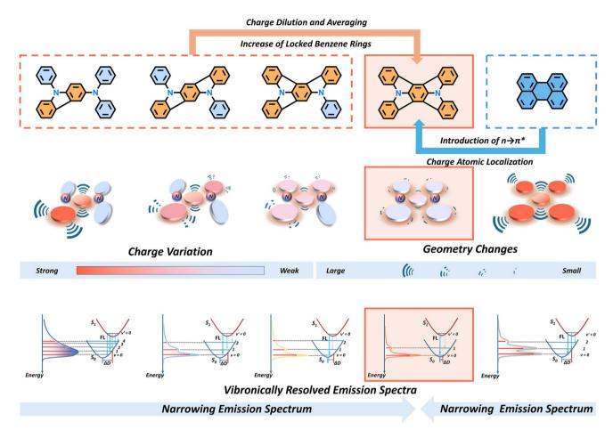
Fig. 5 Mechanism of emission spectrum narrowing.
