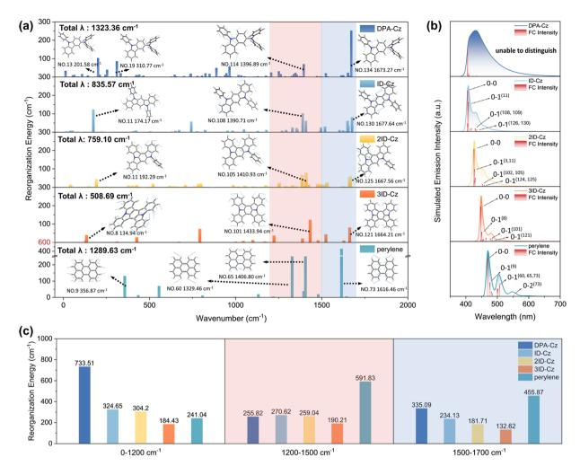
Fig. 4 (a) Reorganization energy *versus* normal-mode frequency at the  $S_0$  potential energy surface, and the high-frequency region is highlighted in the range of  $1200-1700~\text{cm}^{-1}$  for clarity. (b) Simulated vibronically resolved emissions spectra of DPA-Cz, ID-Cz, 2ID-Cz, 3ID-Cz, and perylene. (c) The total  $\lambda$  in  $0-1200~\text{cm}^{-1}$  (white background),  $1200-1500~\text{cm}^{-1}$  (red background) and  $1500-1700~\text{cm}^{-1}$  (blue background) frequency region.
