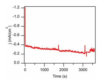
Fig. 4 Controlled potential photoelectrolysis (CPPE) of the stirred solution at  $E_{\rm app}=-1.31$  V vs. Fc<sup>+/0</sup> over 3600 s. CPPE recorded in divided electrolysis cell at 100 mV s<sup>-1</sup> in 100 mM [NBu<sub>4</sub>][PF<sub>6</sub>] 95:5 CH<sub>3</sub>CN: H<sub>2</sub>O solution with a p-Si-CH<sub>3</sub> photoelectrode, Pt mesh counter electrode (in separate compartment), and 10 mM Ag/AgNO<sub>3</sub> reference electrode with AM1.5G illumination (100 mW cm<sup>-2</sup>).
