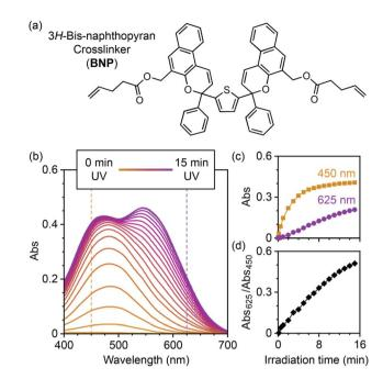
Fig. 2 (a) Structure of the 3H-bis-naphthopyran crosslinker (BNP) used in this study. (b) UV-vis absorption spectra acquired during the photoirradiation (311 nm, 15 min) of a solution of BNP in THF (8  $\mu$ g mL $^{-1}$ , 30 mM BHT, -78 °C). (c) Absorbance at 450 nm and 625 nm as a function of photoirradiation time. (d) Ratio of the absorbance at 625 nm and 450 nm as a function of photoirradiation time.
