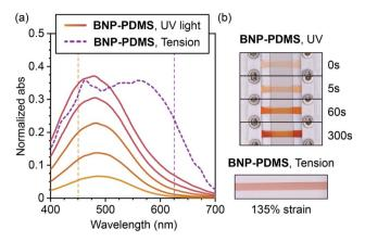
Fig. 4 (a) Absorption spectra of BNP-PDMS after 5 s, 30 s, 60 s, 120 s, and 300 s of photoirradiation with 311 nm UV light compared to a sample of BNP-PDMS at 135% strain. (b) Photographs of BNP-PDMS after 0 s, 5 s, 60 s, and 300 s of photoirradiation with UV light compared to a sample of BNP-PDMS at 135% strain
