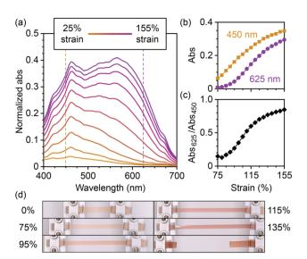
Fig. 3 (a) Normalized UV-vis absorption spectra acquired during uniaxial tensile loading of BNP-PDMS. (b) Absorbance at 450 nm and 625 nm as a function of strain. (c) Ratio of the absorbance at 625 nm versus 450 nm as a function of strain. (d) Photographs of a separate sample of BNP-PDMS at various strain values. The sample failed between 135 and 140% strain.
