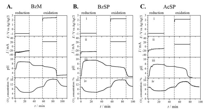
Fig. 3 H-cell CO<sub>2</sub> capture/release tests. (A-C) CO<sub>2</sub> capture/release results in the H-cell, (A) BzM, (B) BzSP, (C) AcSP. Furnasep AEM was used for BzM, and Nafion CEM was employed in the test of BzSP and AcSP. The pyridinium mediators were reduced using a constant potential and were reoxidized using a constant current. (i) Applied potential on the Pt WE, (ii) current of the Pt WE, (iii) pH of electrolyte in the WE compartment and (iv) CO2 concentration in the gas outlet.
