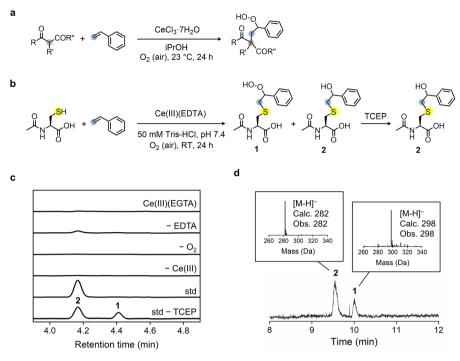
Fig. 1 Ce(iii)-mediated oxidative coupling. (a) Previously reported oxidative reaction of 1,3-dicarbonyl compounds with styrene. Adapted from ref. 27. (b) Oxidative thiol-ene coupling of N-acetylcysteine (NAC) with styrene. (c) HPLC analysis. (d) LC-MS analysis of the products from the reaction shown in b before TCEP treatment.
