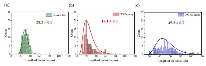
Fig. 6 Comparison of the length of tactoids formed in the aqueous solution with 1% UPy-Gly, 0.9% dextran,  $0.25 \times PBS$ , pH = 7.5 in (a) glass holder, (b) NON- and (c) ON-resonance cavities.
