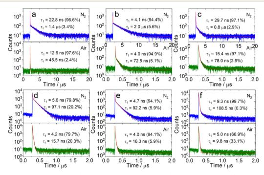
Fig. 3 Fluorescence decay traces of (a) PTZ-DTO at 560 nm, (b) PSeZ-DTO at 550 nm, (c) DPTZ-DTO at 580 nm, (d) PTZ-O-DTO at 400 nm, (e) PTZ-O2-DTO at 410 nm and (f) DPTZ-O-DTO at 470 nm under different atmospheres ( $N_2$  and air).  $\lambda_{ex} = 340$  nm,  $c = 1.0 \times 10^{-5}$  M in TOL, 25 °C.
