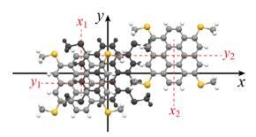
Fig. 4 Definition of mutual positions of molecules in the solid state. The first molecule (black in colour) is placed at the origin on the xy-plane of the Cartesian system so that the molecular long axis aligns with the x-axis, and the positions of the  $\pi$ -stacking molecules are defined by the coordinates of the center of gravity of the molecules. The y-axis projection (top) and the z-axis projection (bottom).
