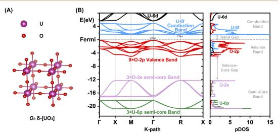
Fig. 1 Geometric and electronic structure of  $\delta$ -[UO<sub>3</sub>]. (A) Geometric structure. (B) Electronic band structure and partial atomic orbital density of states (pDOS). Energy range of semi-core U-6p (green) and O-2s (lilac), and of valence O-2p (red), U-5f (blue) and U-6d (black). SR Kohn-Sham PBE approximation; energies in eV w. r. t. the lower Fermi edge.
