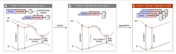
Scheme 5 Proposed design strategy and working mechanism. S<sub>0</sub> – ground state; ICT – intramolecular charge transfer; LE – locally excited; TICT – twisted intramolecular charge transfer.
