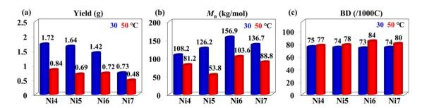
Fig. 2 Comparison of the yield (a), molecular weight (b), and branching density (c) of polyethylene generated using Ni4-Ni7 at 30 and 50 °C.
