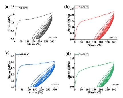
Fig. 4 Plots of hysteresis experiments of ten cycles at 300% strain for polyethylenes generated using Ni1-Ni4 at 30 °C (a-d).
