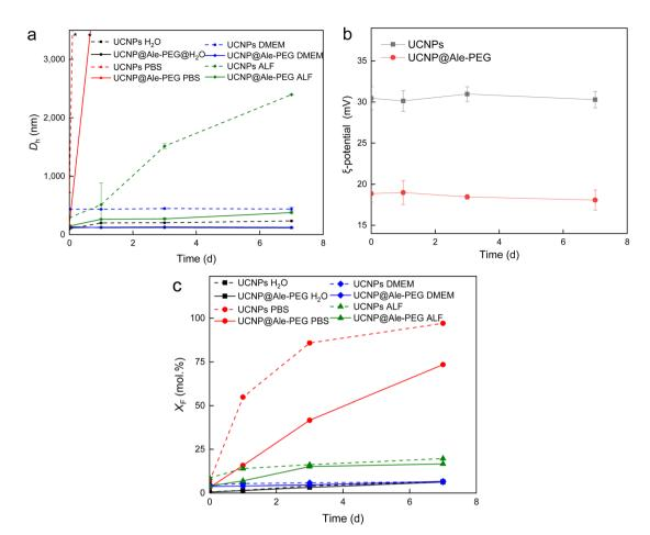
Fig. 5 Time dependencies of (a) hydrodynamic diameter  $D_h$  in water, PBS, DMEM and ALF, (b) ζ-potential of UCNPs and UCNP@Ale-PEG nanoparticles in water and (c)  $F^-$  ion molar fraction ( $X_F$ ) in the supernatants after incubation of particles in water, PBS (pH 7.4), DMEM and ALF at 37 °C. \* Beyond the scope of measurement.
