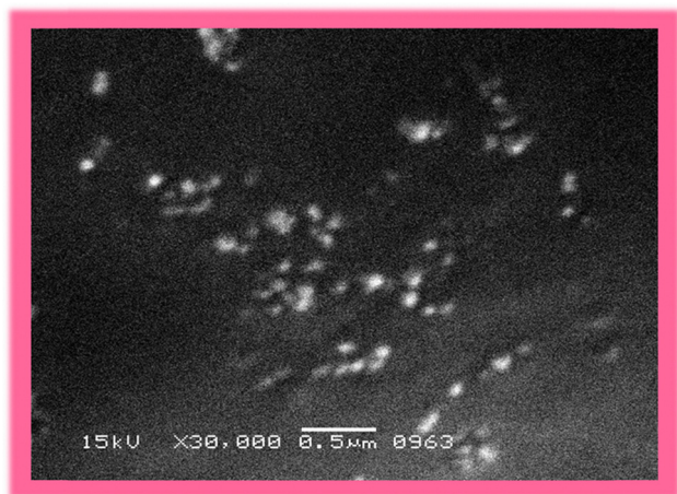
Fig. 21 SEM microphotograph of diclofenac -capped silver NPs ( 1a ) obtained by direct reaction of silver I nitrate and dh (molar ratio 1:2) in methanol upon stirring at 45 °C.
