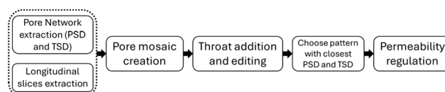
Fig. 1 Proposed steps for rock pattern design method.
