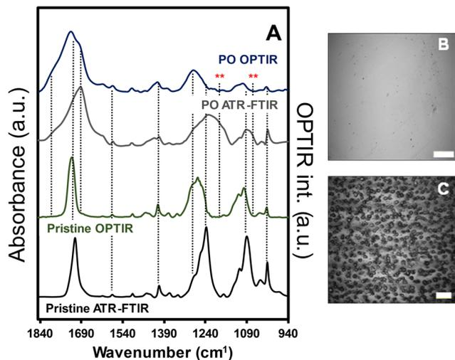
**Fig. 1** A) Normalized ATR-FTIR and OPTIR spectra of PET films prior to (pristine) and after exposure at <10% relative humidity. Optical images of film surface in the B) absence and C) presence of saturated relative humidity during exposure. The scale bars for panels B and C are 40  $\mu\text{m}$  and 10  $\mu\text{m}$ , respectively. The red asterisks (\*\*) represent the vibrational modes observed with ATR-FTIR that were not present in the OPTIR spectra.
