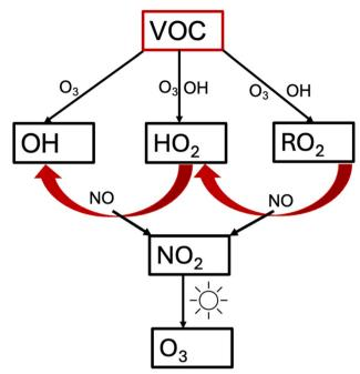
Fig. 6 Reactions following oxidation of VOCs indoors:  $HO_2$ : hydroperoxy radical;  $RO_2$ : generic term for organic peroxy radicals; NO: nitric oxide;  $NO_2$ : nitrogen dioxide;  $O_3$ : ozone; OH: hydroxyl radical; VOC: volatile organic compounds.
