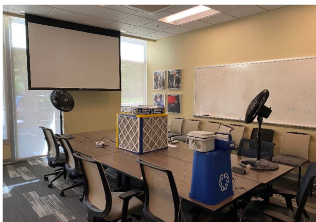
Fig. 1 CR box experimental test setup in a conference room.
