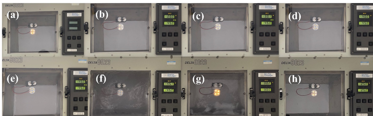
Fig. 4 Photographs of the bulbs lit by LFP|Li + @Ni-MOF|Li cells at different temperatures: (a) RT, (b) −20 °C, (c) −30 °C, (d) −40 °C, (e) and (f) −45 °C, (g) 30 °C, and (h) 25 °C.
