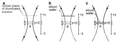
Fig. 48 (a) Illustration of the contribution to  $I_{Raman}$  from a certain plane of illuminated solution. (b) and (c) Illustration of vertical movement of a flat Si waver for obtaining the confocal depth dependence of the Raman signal. Reproduced from ref. 402 with permission. Copyright 1998 Elsevier.
