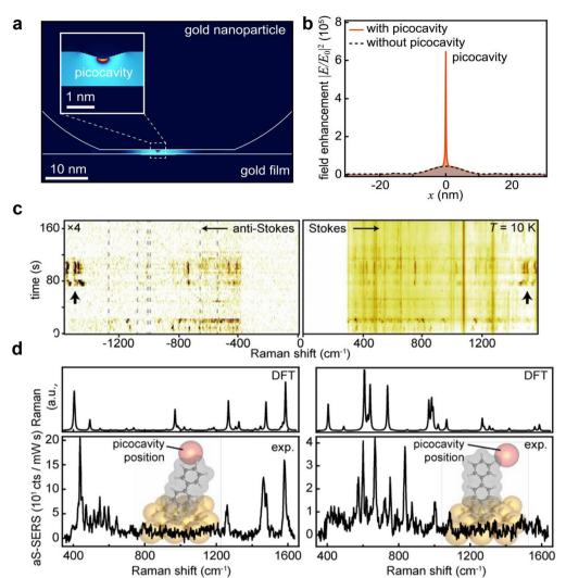
Fig. 38 (a) The schematics of picocavity formed by adatoms on Au nanoparticles. (b) Near field enhancement in the cavity, (c) Time-series anti-Stokes and Stokes SERS in the picocavity. (d) Comparison of two experimental spectra (bottom) with DFT simulated spectra (top) under the assumption of atomic-scale field confinement (inset shows geometries, red sphere shows field ocalization for simulations). Figures are reproduced from ref. 358 with permission. Copyright 2016 AAAS
