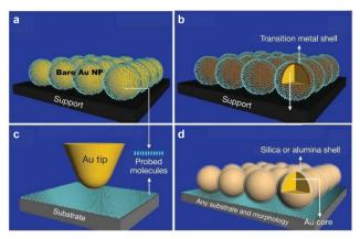
Fig. 47 Schematic of the mode of SERS, TERS, and SHINERS. (a) Bare Au nanoparticles: contact mode. (b) Au core-transition metal shell nanoparticles adsorbed by probed molecules: contact mode. (c) TERS: noncontact mode. (d) SHINERS: shell-isolated mode. Figures are reproduced from ref. 20 with permission. Copyright 2010 Springer Nature.
