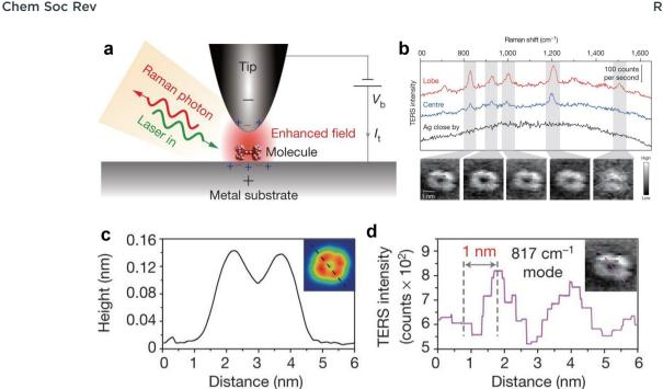
Fig. 36 (a) Schematic of single-molecule TERS at LT-UHV condition. (b) The typical Raman spectrum taken from different positions of molecules. (c) Height profile of a line trace in the inset STM topograph. (d) TERS intensity profile of the same line trace for the inset Raman map associated with the 817 cm<sup>-1</sup> Raman peak. Figures are reproduced from ref. 354 with permission. Copyright 2013 Springer Nature
