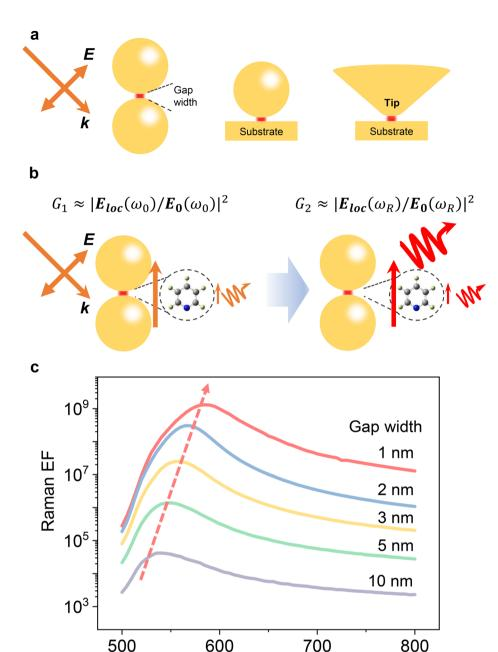
Fig. 23 (a) Representative nanostructures for gap-mode SERS/TERS, including nanoparticle dimer, nanoparticle on substrate and tip on substrate (b) The two-step process of enhancement of the electromagnetic field in SERS for nanoparticle dimer. (c) The spectra of the maximum Raman EFs for nanoparticle dimers with different gap widths.
