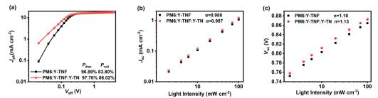
Fig. 4 (a)  $J_{ph}-V_{eff}$  curves, (b)  $J_{sc}-P_{light}$  and (c)  $V_{oc}-P_{light}$  of the binary device based on PM6:Y-TNF and the ternary device based on PM6:Y-TNF (1:1:0.1, w/w/w).
