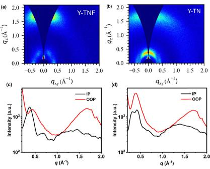
Fig. 2 (a) The two-dimensional GIWAXS patterns of Y-TNF pure film, (b) the two-dimensional GIWAXS patterns of Y-TN pure film, (c) the corresponding in-plane and out-of-plane profiles under Y-TNF pure film optimal conditions, and (d) the corresponding in-plane and out-of-plane profiles under Y-TN pure film optimal conditions.
