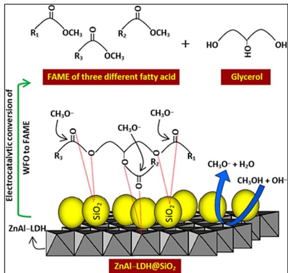
Fig. 10 Suggested mechanism of the transesterification process using the ZnAl/LDH-SiO 2 composite.
