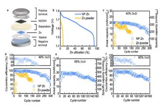
Fig. 3 (a) Schematic of Zn II NiOOH coin cell. (b) Various anodes for zinc are used in primary Zn II NiOOH alkaline anodes. (c) Cycle number vs. discharging capacities of NP Zn and Zn powder sample. (d) Coulombic efficiency of NP Zn and Zn powder at 40% DoD. (e) At 60% depth of DoD, discharging capacities of the NP Zn anodes. (f) Coulombic efficiency of the sample at 60% DoD
