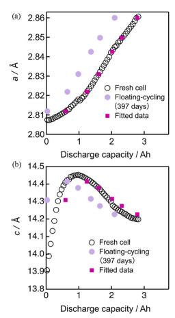
Fig. 9 Least squares fitting results of the lattice constants (a) a and (b) c for the cell after 397 days of floating-cycling.
