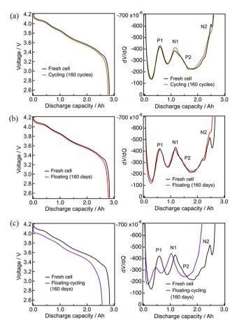
Fig. 2 Discharge curves and dV/dQ curves after 160 cycles: (a) cycling, (b) floating, (c) floating-cycling
