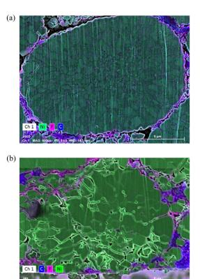
Fig. 12 EDX results of positive electrode cross section (electrolyte side): (a) fresh cell and (b) floating-cycling
