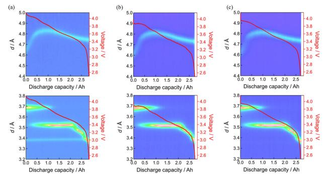
Fig. 5 Neutron diffraction patterns of 003 diffraction of positive electrode (upper) and 001 diffraction of negative electrode (lower): (a) fresh cell, (b) floating after 160 days, (c) floating after 397 days.
