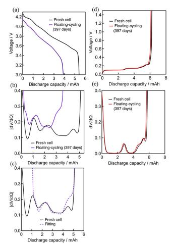
Fig. 10 Discharge curves and dV/dQ curves of the half cells with the electrodes of fresh cell and floating-cycling: (a) discharge curves of positive electrode, (b) dV/dQ curves of positive electrode, (c) fitting results, (d) discharge curves of negative electrode, (e) dV/dQ curves of negative electrode
