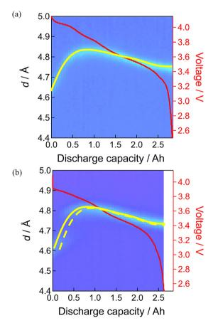
Fig. 7 Line broadening of neutron diffraction patterns of 003 diffraction of positive electrode: (a) fresh cell, (b) floating-cycling after 160 days.
