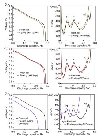
Fig. 3 Discharge curves and dV/dQ curves after 397 cycles: (a) cycling (b) floating, (c) floating-cycling
