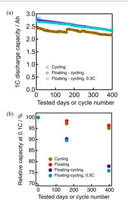
Fig. 1 (a) Trends of 1C discharge capacity of vertically-set cells as function of tested days (floating and floating-cycling) and cycle number (cycling) (b) The corresponding capacity retention at 0.1C after 160 and 397 days or cycles. The state of health check was employed after 160 cycles as shown below, which caused some capacity recovery in cycling.
