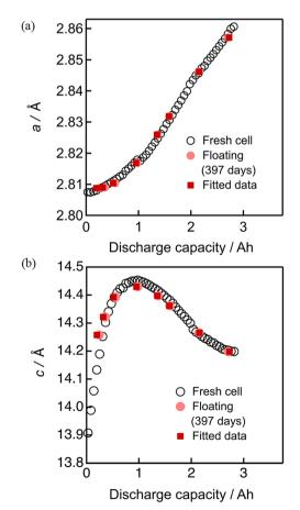
Fig. 8 Least squares fitting results of the lattice constants (a) a and (b) c for the cell after 397 days of floating
