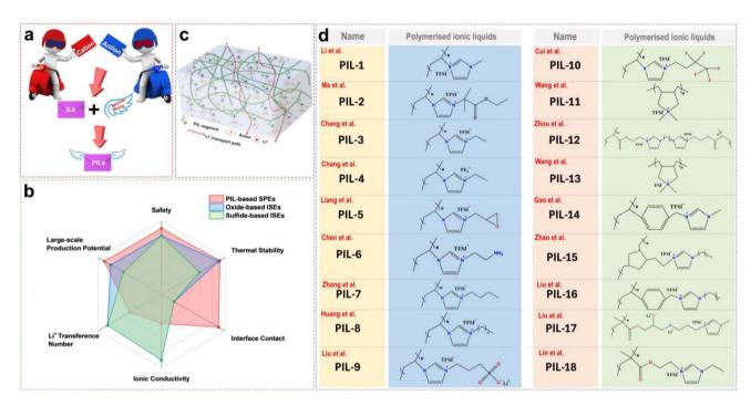
Fig. 9 (a) Schematic illustration of the relationship between ILs and PILs. (b) Comparison of the main properties of solid-state electrolytes using PIL-based SPEs, oxide-based inorganic solid-state electrolytes (ISEs), and sulfide-based ISEs in a radar chart. (c) Schematic illustration of PILbased solid-state electrolyte transport model. (d) Summary of the chemical structures of the PILs used for solid-state electrolytes.
