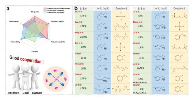
Fig. 7 (a) Comparison of the physicochemical and electrochemical properties of ILEs using an ether-based cosolvent, an ester-based cosolvent, and a locally concentrated cosolvent in a radar chart; and classical LCILE solvation structure. (b) Summary of the combination and collocation of LCILE composed of a lithium salt, cosolvent and ILs.
