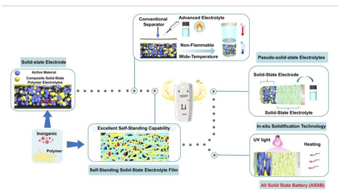
Fig. 17 Schematic illustration of solidified electrodes for applications in liquid and solid-state electrolytes.
