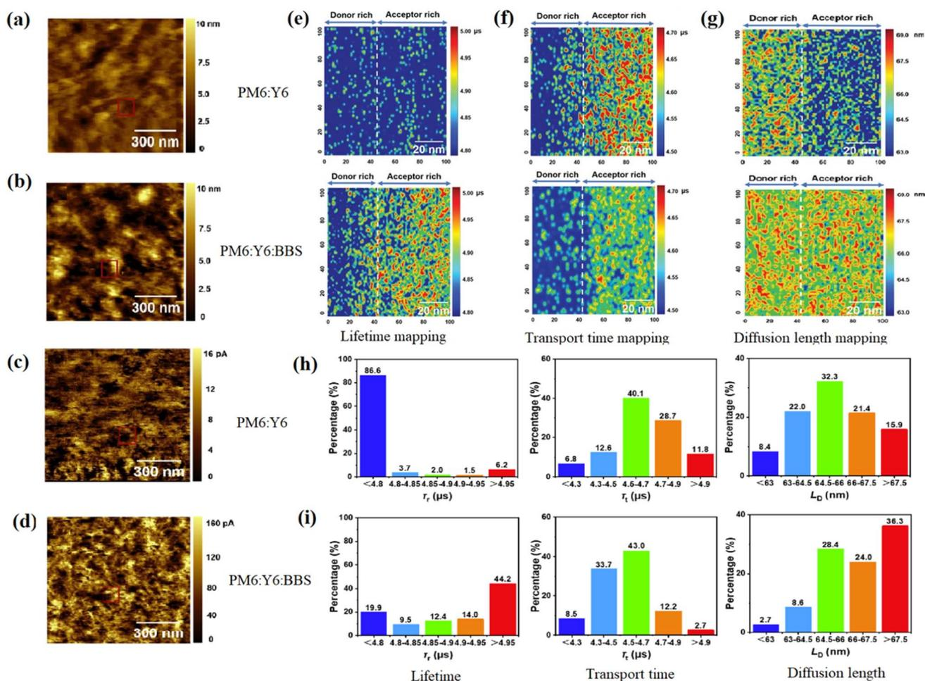
Fig. 4 AFM-topography of (a) PM6:Y6, and (b) PM6:Y6:BBS. *c*-AFM-conductivity of (c) PM6:Y6 and (d) PM6:Y6:BBS. (e) Carrier lifetime ' $\tau_t$ ', (f) carrier transport time ' $\tau_r$ ', (g) carrier diffusion length  $L_D$ . (h and i) Statistical distribution of  $\tau_t$ ,  $\tau_r$ , and  $L_D$  for PM6:Y6 and PM6:Y6:BBS organic films.<sup>60</sup> Reproduced from ref. 60 with permission from John Wiley and Sons, copyright 2022.
