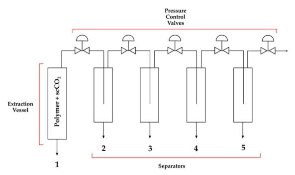
Fig. 6 Schematic setup of an extractor for isothermal decreasing pressure profiling of a polymer (the figure is a free adaptation from a generic extractor scheme).
