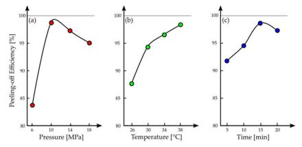
Fig. 10 Effect of (a) pressure, (b) temperature and (c) time on the exfoliation efficiency with  $scCO_2$ . All graphics adapted from the work of Mu et al.<sup>74</sup> with permission from John Wiley and Sons.
