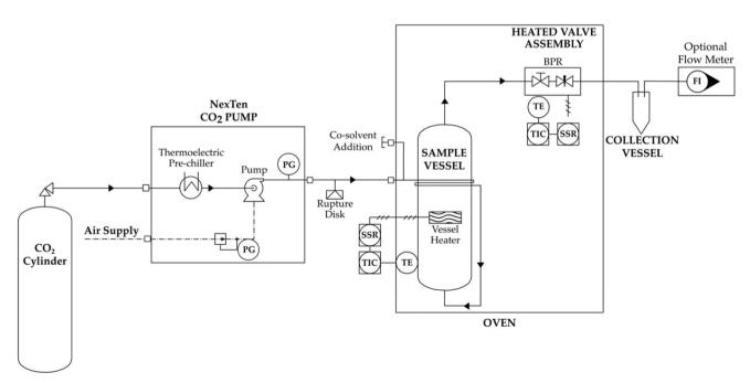
Fig. 4 Scheme of a lab-scale SFT-120 extractor from Supercritical Fluid Technologies, Inc.
