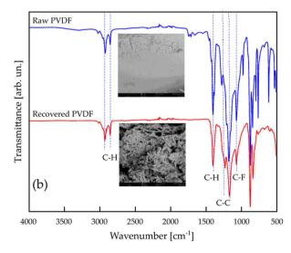
Fig. 9 Characterization of the PVDF recovered by Fu et al. (red plots) and comparison with raw PVDF (blue plots) as a reference by means of (a) TGA and (b) FT-IR analyses (adapted from ref. 122. Y. Fu, J. Schuster, M. Petranikova and B. Ebin, Resour., Conserv. Recycl., 2021, 172, 105666. No permission required. License: CC BY 4.0, Elsevier).
