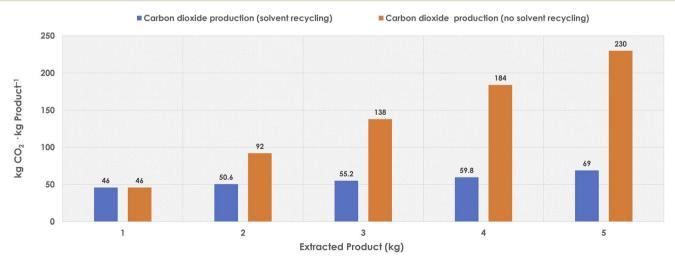
Fig. 2 Assessment of the CO<sub>2</sub> production during an extractive downstream from a DES media, using an organic solvent, and reusing it for several cycles. Data assumed for extracting 10 L of DES, to produce 1 kg product at 100 g substrate per LDES, and that two-fold volume of extractive solvent is used (20 L). 10% of solvent loss is assumed between each cycle.
