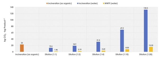
Fig. 4 Obtained TCRs (kg CO<sub>2</sub> per kg product) when treating 10 L DES as expended reaction media (needed to produce 1 kg product at 100 g substrate per L<sub>DFS</sub>), and following different options such as organic incineration, or different aqueous dilution ratios and establishing water incineration or mild wastewater treatment (WWTP). Calculations based on TCR methods retrieved from literature. 43,45,46
