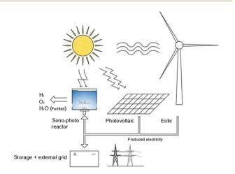
Fig. 8 Sono-photolysis technology integration in existing renewable production systems. The synergistic production of hydrogen, oxygen and purified water is highlighted as a key parameter for the application of this technology.
