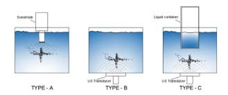
Fig. 4 Common configuration of a sonoreactor
