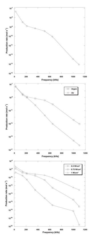
Fig. 6 Hydrogen production as a function of frequency, atmosphere and intensity.<sup>70</sup>
