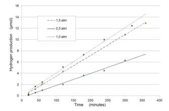
Fig. 5 Hydrogen production rates during exposition time, changing the rector inner pressure.87
