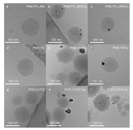
Fig. 3 Bright-field cryo-TEM images of NPs showing their structures and the differences in cocatalyst deposition: (a), (d) and (g), pristine organic NPs of different composition with D: A weight ratio 1:1; (b), (e) and (h), corresponding NPs with Ag cocatalyst; (c), (f) and (i), corresponding NPs with Au cocatalyst. Note: the dark contrast in the corners of the images (b), (d), (e), and (g) arises from the carbon TEM grid. Additional images and their analysis are shown in Fig. S8-S16.†
