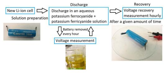
Fig. 1 The experimental measurement setup and procedure for the battery voltage behaviour.
