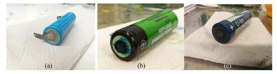
Fig. 10 Corrosion of the battery poles after discharging experiments: (a) Panasonic battery with junction plates at the terminals, (b) Biltema battery, and (c) Ansmann battery.
