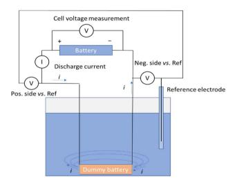
Fig. 2 Schematic of the measurement system.
