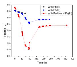
Fig. 3 Internal electrochemical discharge of Panasonic LIBs in individual 5 wt% potassium hexacyanoferrate(II) and 5 wt% potassium hexacyanoferrite(III) and in an electrolyte containing a 5 wt% solution of potassium hexacyanoferrate and potassium hexacyanoferrite.
