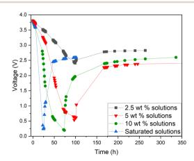
Fig. 5 Electrochemical discharge of a Panasonic LIB in a redox electrolyte containing potassium hexacyanoferrate(II) and potassium hexacyanoferrite(III) in different concentrations from 2.5 wt%, 5 wt%, 10 wt% to saturation solution.
