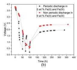
Fig. 6 (a) Discharge behaviour of Panasonic LIBs with varying discharge times. (b) Comparison of periodic and non-periodic discharge of a Panasonic LIB; both experiments were conducted in a redox electrolyte containing a 5 wt% solution of potassium hexacyanoferrate and potassium hexacyanoferrite.
