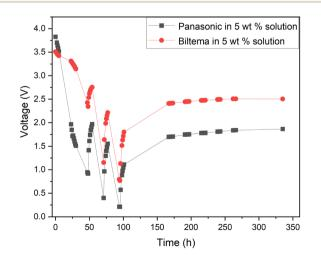
Fig. 12 Comparison of the periodic discharge of Panasonic and Biltema LIBs in a redox electrolyte containing a 5 wt% solution of potassium hexacyanoferrate and potassium hexacyanoferrite.
