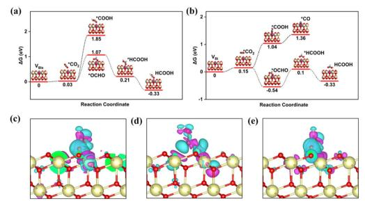
Fig. 2 Free energy profile for the CRR on  $V_{Bi}$  (a) and  $V_{Bis}$  (b) with various intermediates. Electron density difference plots for \*OCHO (c), \*COOH (d) on  $V_{Bi}$ , and \*COOH (d) on  $V_{Bis}$ . The isosurface value was set to 0.003 e Å<sup>-3</sup>. The charge accumulation and loss are shown in the cyan and pink regions, respectively. Black represents C.
