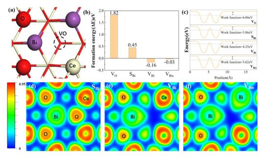
Fig. 1 (a) Configuration of four concept structures in CeO<sub>2</sub> (111). The formation energy (b), work function (c), and electron localization function (d-f) of the above four materials. White, red, and purple represent Ce, O, and Bi, respectively
