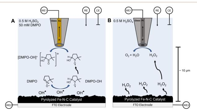
Scheme 1 SECM substrate generation—tip collection (SG/TC) for OH\* detection using DMPO and for H<sub>2</sub>O<sub>2</sub> detection. (A) Schematic depiction of substrate-generated OH\* detection using the DMPO spin trap with a 25 µm diameter gold ultramicroelectrode as the tip biased to oxidize the DMPO-OH adduct. (B) A depiction of the SECM H<sub>2</sub>O<sub>2</sub> detection experiment using a platinum UME biased to perform H<sub>2</sub>O<sub>2</sub> oxidation.
