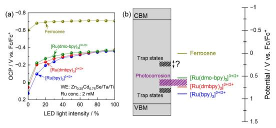
Fig. 5 (a) OCPs of the  $Zn_{0.25}Cd_{0.75}Se$  photoanode in the acetonitrile electrolyte containing equal molar amounts of  $Ru^{2+}$  and  $Ru^{3+}$  complexes with the total concentration of 2 mM and 0.1 M TBAPF<sub>6</sub> as functions of light intensity. Various intensities of 600 nm monochromatic light from the LED were used as light sources. (b) Schematic energy diagram of the band structure of  $Zn_{0.25}Cd_{0.75}Se$  accompanied by the potentials for trap sites and photocorrosion.
