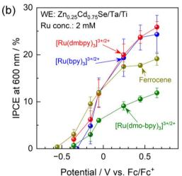
Fig. 3 (a) IPCE spectra of the  $Zn_{0.25}Cd_{0.75}Se$  photoanode under an applied potential of 0.45 V vs. Fc/Fc<sup>+</sup>, and (b) IPCE–potential curves for the photoanode under illumination by 600 nm monochromatic light emitted from a Xe lamp. The acetonitrile electrolyte contained equimolar amounts of  $Ru^{2+}$  and  $Ru^{3+}$  complexes with a total concentration of 2 mM and 0.1 M TBAPF<sub>6</sub>.
