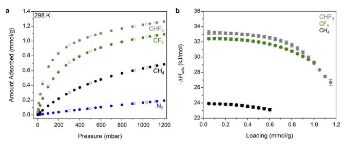
Fig. 3 (a) Adsorption isotherm data for  $CHF_3$ ,  $CF_4$ ,  $CH_4$ , and  $N_2$  in Zn(fba) at 298 K. Filled and open symbols correspond to adsorption and desorption points, respectively. (b) Differential enthalpy of adsorption as a function of loading for  $CHF_3$ ,  $CF_4$ , and  $CH_4$ . Error bars are shown for all data points.
