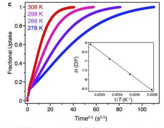
Fig. 6 (a) SEM image of sieved Zn(fba) showing a wide dispersity of crystallite sizes. (b) Transient adsorption data for CF<sub>4</sub> (green) or CHF<sub>3</sub> (grey) adsorption in Zn(fba) following a 1.00 mmol g<sup>-1</sup> dose at 298 K. (c) Variable temperature CF<sub>4</sub> transient adsorption data from which values of  $D/l^2$  were calculated. The inset shows the Arrhenius plot from which the activation energy of diffusion was determined.
