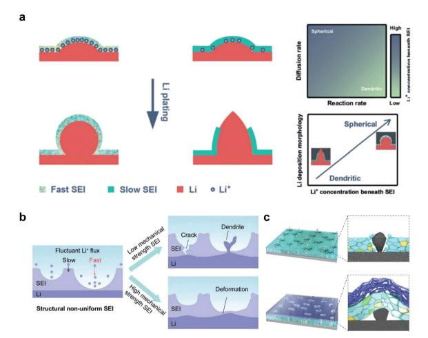
Fig. 4 (a) The diffusion-reaction competition mechanism causing spherical/dendritic Li deposition with fast SEI/slow SEI. (b) Scheme of the morphology evolution in LMBs with a nonuniform SEI. (c) Cracks and distortions of SEI under low and high mechanical strength, respectively.
