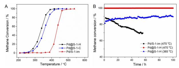
Fig. 3 (A) Catalytic performance of methane combustions over Pd@S-1-H, Pd@S-1-C, and Pd/S-1-im catalysts. Reaction condition: 2% CH<sub>4</sub>-20% O<sub>2</sub>-78% N<sub>2</sub>, gas hourly space velocity (GHSV) =  $36\,000$  mL  $g_{cat}^{-1}$  h<sup>-1</sup>. (B) Long-term stability of methane combustions over Pd@S-1-H and Pd/S-1-im catalysts with a GHSV of  $36\,000$  mL  $g_{cat}^{-1}$  h<sup>-1</sup>.
