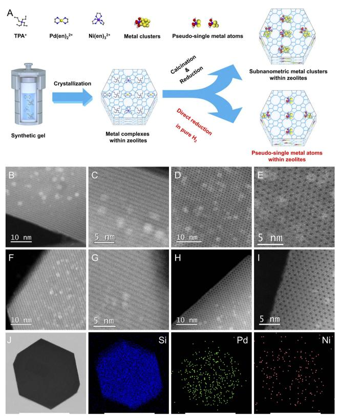
Fig. 1 (A) Schematic illustration of the preparation of zeolite-encaged Pd-based catalysts. C<sub>s</sub>-corrected STEM images of (B and C) Pd@S-1-C; (D and E)  $0.8Pd0.2Ni(OH)_2@S-1-C$ ; (F and G) Pd@S-1-H; (H and I)  $0.8Pd0.2Ni(OH)_2@S-1-H$ . (J) TEM image of  $0.8Pd0.2Ni(OH)_2@S-1-H$  catalyst and corresponding EDX mapping images for Si, Pd, and Ni elements. Scale bar: 250 nm.
