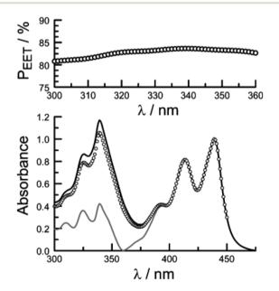
Fig. 8 The lower panel shows a comparison of normalised absorption (black curve) and excitation (open circles) spectra recorded for PY-P<sub>8</sub>-PER in dilute chloroform solution. The fluorescence wavelength was 525 nm. The grey curve represents the absorption spectrum derived for the perylene component of the dyad. The upper panel shows the wavelength dependence for  $P_{\rm EET}$  as measured by this procedure, the median value being 83%.
