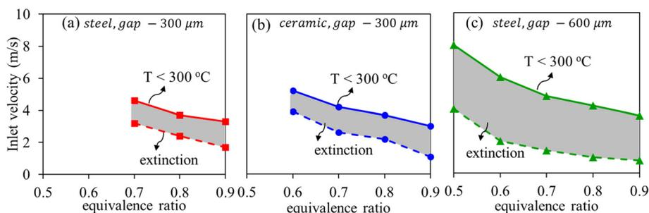
**Fig. 12** Comparison of the operating regimes of the integrated device for (a) steel/ $300 \mu\text{m}$ ; (b) ceramic/ $300 \mu\text{m}$ ; and (c) steel/ $600 \mu\text{m}$ , where steel or ceramic represent material of the inner wall and the number represents the gap-size of the outer recirculation channels. The lower branch (dashed lines) indicates the extinction limit and the upper branch (solid lines) indicates the velocities that limit the skin temperatures below  $300^\circ\text{C}$ .
