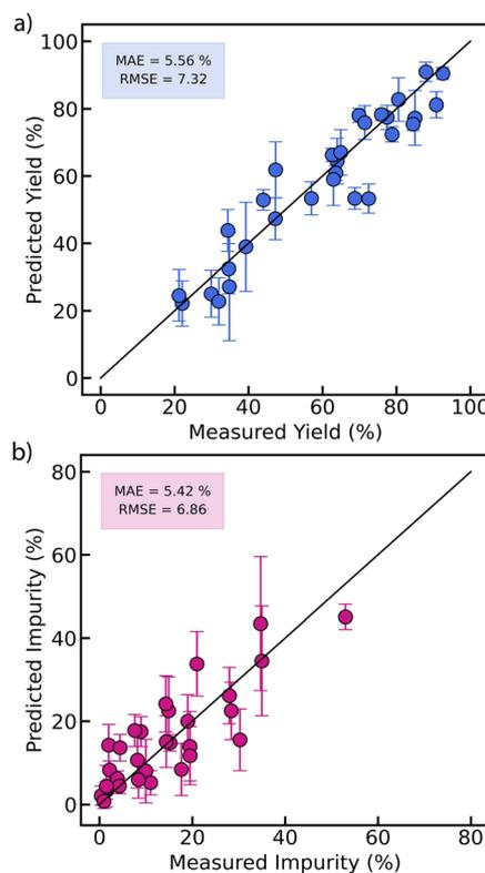
**Fig. 6** Yield (a) and impurity (b) predictions of 30 experimental conditions unseen by the Gaussian process (GP) surrogate model of the first optimization campaign (Fig. 2). The mean (data points) and the standard deviation (error bars) of the predictions were calculated from the average of 1000 samples drawn from the GPs. Black solid line represents the parity line.
