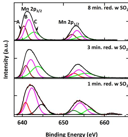
Fig. 19 Mn 2p spectra of samples reduced for 1, 3 and 8 minutes for 1 cycle at 900 °C with 9% CH<sub>4</sub>-5000 ppm SO<sub>2</sub>-balance N<sub>2</sub>.
