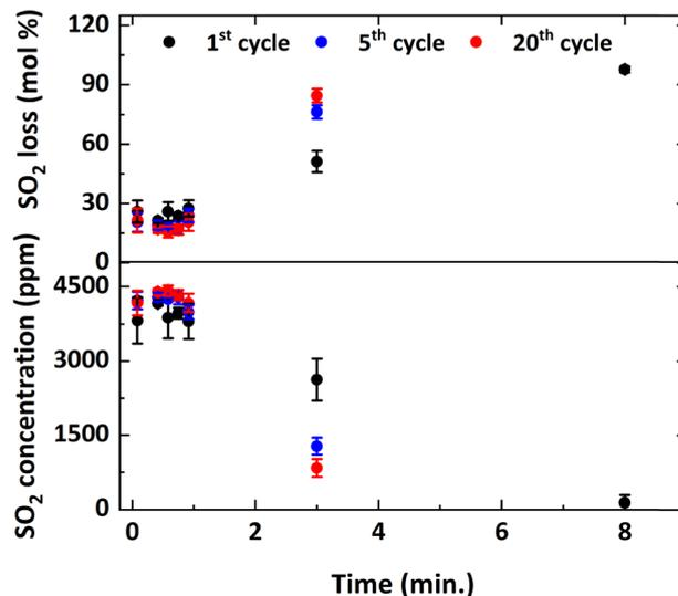
Fig. 7 Measured SO<sub>2</sub> concentration profile and calculated SO<sub>2</sub> loss (mol%) as a function of reduction period for the 1st, 5th, and 20th cycles at 900 °C with 9% CH<sub>4</sub>-5000 ppm SO<sub>2</sub>-balance N<sub>2</sub>.
