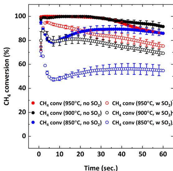
Fig. 11 CH<sub>4</sub> conversion as a function of reduction period during the 5th cycle with 9% CH<sub>4</sub>-balance N<sub>2</sub> and 9% CH<sub>4</sub>-5000 ppm SO<sub>2</sub>-balance N<sub>2</sub> at different temperatures (850, 900, 950 °C).
