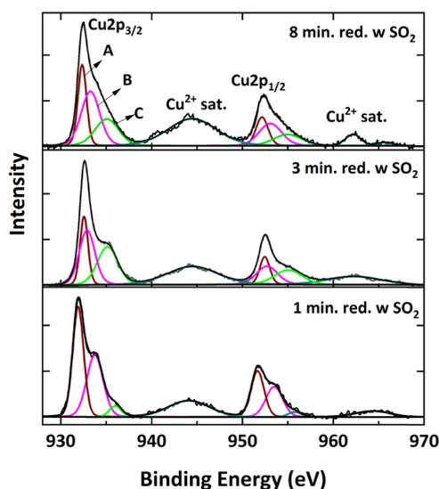
Fig. 18 Cu 2p spectra of samples reduced for 1, 3 and 8 minutes for 1 cycle at 900 °C with 9% CH<sub>4</sub>-5000 ppm SO<sub>2</sub>-balance N<sub>2</sub>.
