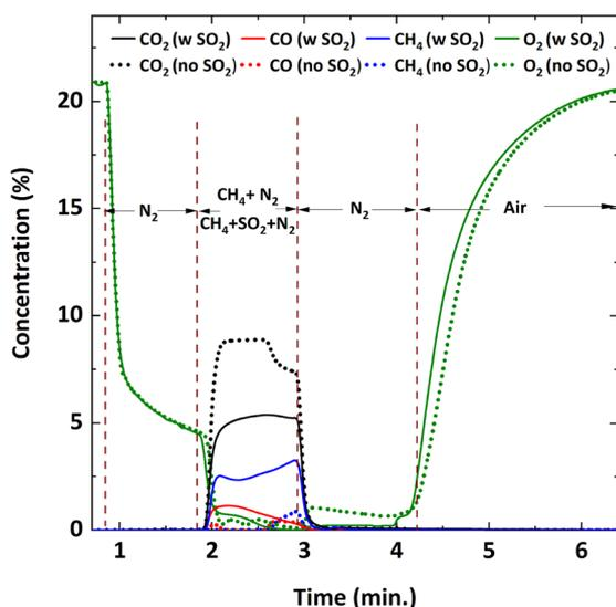
Fig. 3 Flue gas concentration profiles during the 5th cycle at 900 °C with and without 5000 ppm SO<sub>2</sub>. The reducing gas is 9% CH<sub>4</sub>-balance N<sub>2</sub> and 9% CH<sub>4</sub>-5000 ppm SO<sub>2</sub>-balance N<sub>2</sub>. The oxidizing gas is air.
