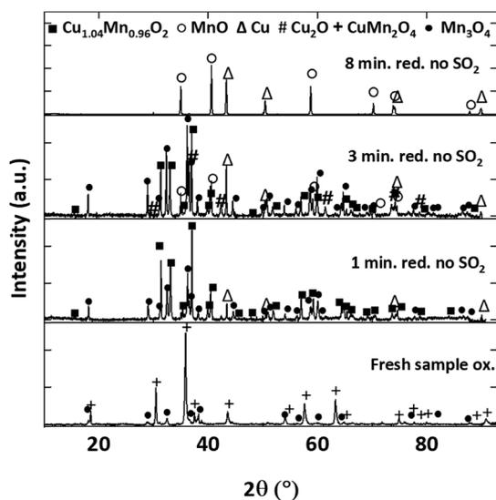
Fig. 15 XRD patterns of samples reduced for 1, 3 and 8 minutes for 5 cycles at 900 °C with 9% CH<sub>4</sub>-balance N<sub>2</sub> and a fresh oxidized sample.
