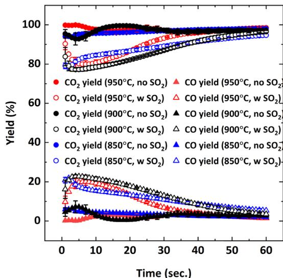
Fig. 12 CO<sub>2</sub> and CO yields as a function of reduction period during the 5th cycle with 9% CH<sub>4</sub>-balance N<sub>2</sub> and 9% CH<sub>4</sub>-5000 ppm SO<sub>2</sub>-balance N<sub>2</sub> at different temperatures (850, 900, 950 °C).
