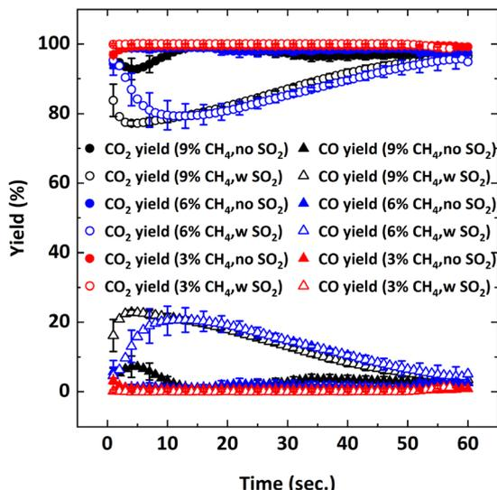
Fig. 9 CO<sub>2</sub> and CO yields as a function of reduction period during the 5th cycle at 900 °C with Y% CH<sub>4</sub>-balance N<sub>2</sub> and Y% CH<sub>4</sub>-5000 ppm SO<sub>2</sub>-balance N<sub>2</sub> where Y: 3, 6, 9.
