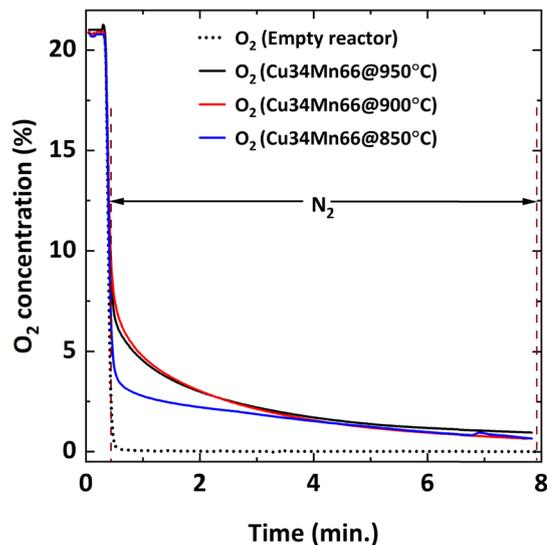
Fig. 13 O<sub>2</sub> concentration profile during oxygen uncoupling of Cu<sub>34</sub>Mn<sub>66</sub> particles at different temperatures (850, 900, 950 °C).
