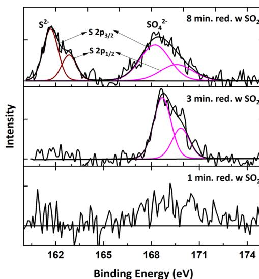
Fig. 17 S 2p spectra of samples reduced for 1, 3 and 8 minutes for 1 cycle at 900 °C with 9% CH<sub>4</sub>-5000 ppm SO<sub>2</sub>-balance N<sub>2</sub>.
