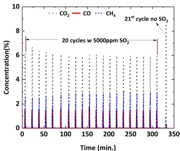
Fig. 14 Multicycle redox behavior of Cu<sub>34</sub>Mn<sub>66</sub> particles at 900 °C with 9% CH<sub>4</sub>-5000 ppm SO<sub>2</sub>-balance N<sub>2</sub>. Reducing time is 1 minute.
