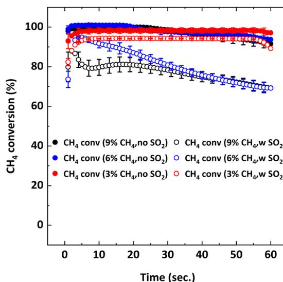
Fig. 8 CH<sub>4</sub> conversion as a function of reduction period during the 5th cycle at 900 °C with Y% CH<sub>4</sub>-balance N<sub>2</sub> and Y% CH<sub>4</sub>-5000 ppm SO<sub>2</sub>-balance N<sub>2</sub> where Y: 3, 6, 9.
