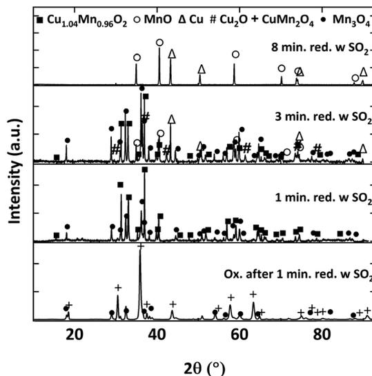
Fig. 16 XRD patterns of samples reduced for 1, 3 and 8 minutes for 5 cycles at 900 °C with 9% CH<sub>4</sub>-5000 ppm SO<sub>2</sub>-balance N<sub>2</sub> and oxidized sample after 1-minute reduction for 5 cycles at 900 °C 9% CH<sub>4</sub>-5000 ppm SO<sub>2</sub>-balance N<sub>2</sub>.
