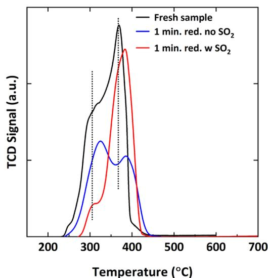
Fig. 20 H<sub>2</sub>-TPR spectra of fresh Cu<sub>34</sub>Mn<sub>66</sub> and samples reduced for 1 minute for 5 cycles at 900 °C with 9% CH<sub>4</sub>-balance N<sub>2</sub> and 9% CH<sub>4</sub>-5000 ppm SO<sub>2</sub>-balance N<sub>2</sub>.
