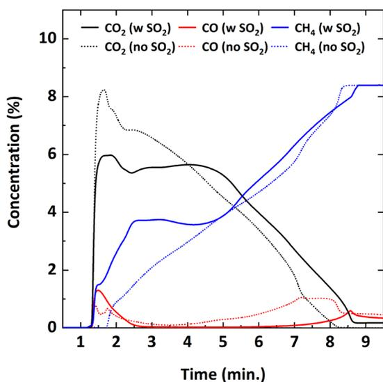
Fig. 6 Flue gas concentration profiles during complete reduction of Cu<sub>34</sub>Mn<sub>66</sub> particles at 900 °C with 9% CH<sub>4</sub>-balance N<sub>2</sub> and 9% CH<sub>4</sub>-5000 ppm SO<sub>2</sub>-balance N<sub>2</sub>.
