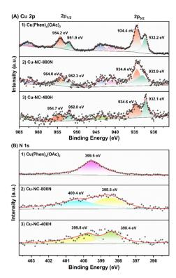
Fig. 5 The XPS of (A) Cu 2p signals: (1) Cu(Phen) $_x$ (OAc) $_2$ , (2) Cu-NC-800N, and (3) Cu-NC-400H samples and (B) N 1s signals: (1) Cu(Phen) $_x$ (OAc) $_2$ , (2) Cu-NC-800N, and (3) Cu-NC-400H samples.
