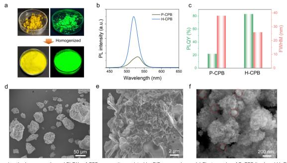
Fig. 3 Improving the homogeneity and PLQYs of CPB composites assisted by SiO<sub>2</sub> nanospheres. (a) Photographs of P-CPB (top) and H-CPB (bottom) under the irradiation of daylight and UV light (right, 365 nm). (b) PL spectra of P-CPB and H-CPB. (c) PLQY value and FWHM of P-CPB and H-CPB. (d) Typical SEM image of P-CPB. (e) High-magnification SEM image of P-CPB. (f) Typical SEM image of H-CPB composites
