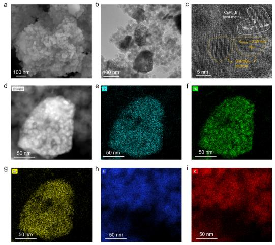
Fig. 2 Microstructural characterization of H-CPB composites. (a) Typical SEM images of H-CPB. (b) SEM images of H-CPB. (c) HRTEM image of CsPbBr<sub>3</sub> NCs embedded in  $CsPb_2Br_5$ . (d)—(i) HAADF-STEM image and the corresponding elemental mapping images showing the elemental distribution of Cs, Pb, Br, Si, and O.
