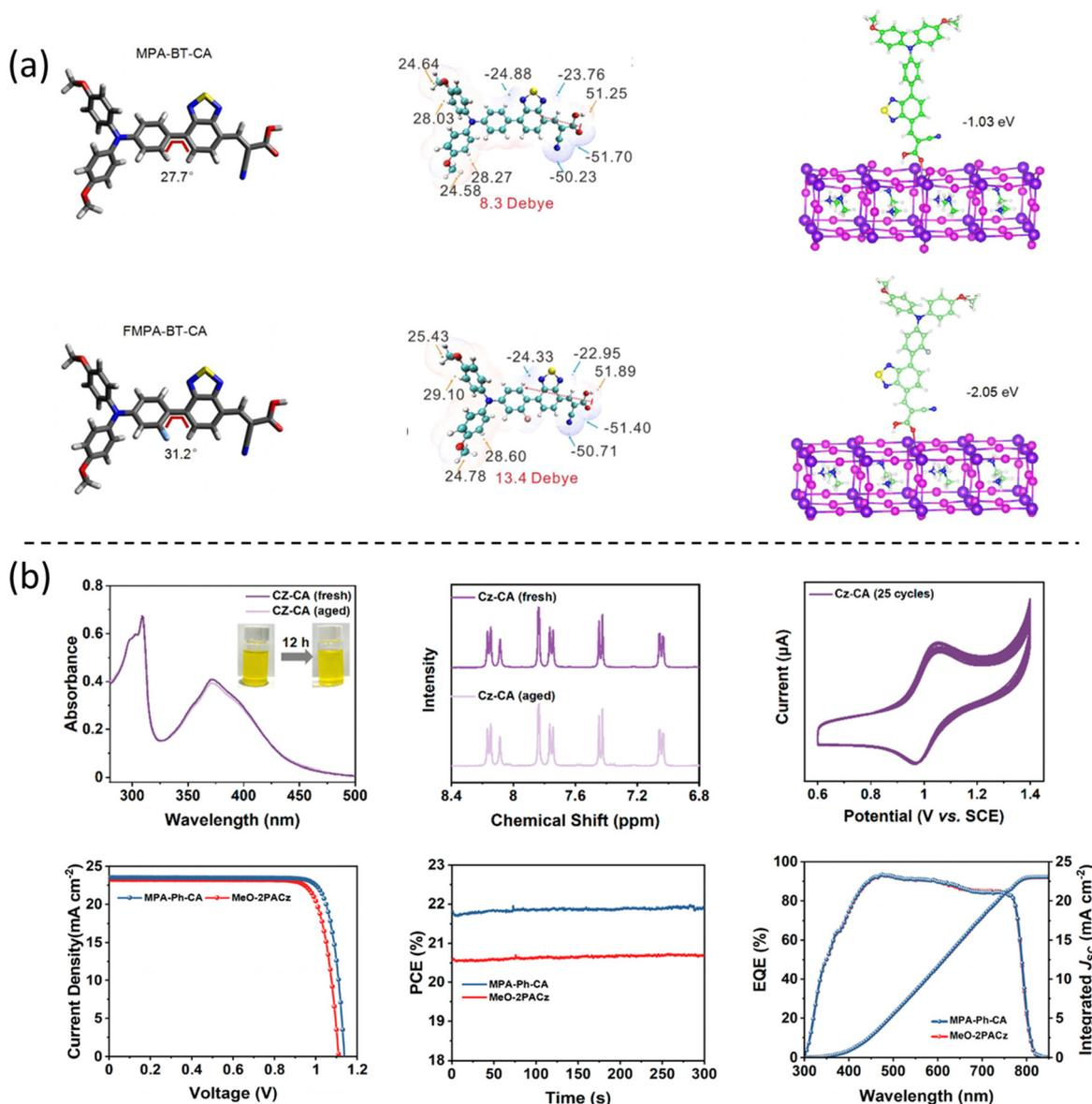
Fig. 10 (a) The calculated dipole moments of the MPA-BT-CA and FMPA-BT-CA SAMs. Reproduced with permission.<sup>45</sup> Copyright 2022, ACS. (b) Measurements to characterize the molecular stability of the CZ-CA SAM and the device performance based on the MPA-Ph-CA molecule. Reproduced with permission.<sup>25</sup> Copyright 2022, ACS.
