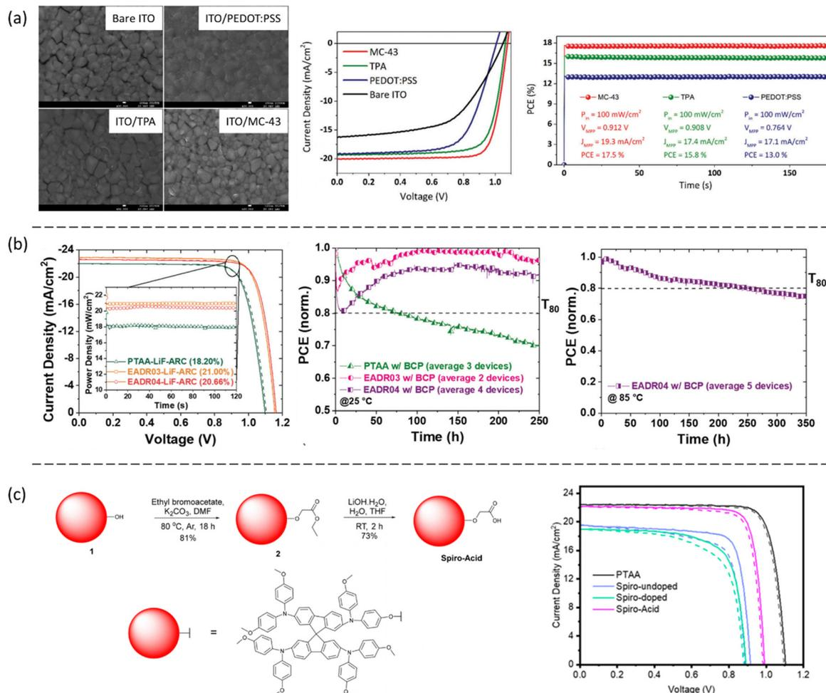
Fig. 4 (a) Morphology of the perovskite deposit onto the TPA and MC-43 SAM layer, and the corresponding device performance. Reproduced with permission.<sup>29</sup> Copyright 2019, RSC. (b) Device performance of EADR03 and EADR04 and their variation with time. Reproduced with permission.<sup>24</sup> Copyright 2021, RSC. (c) The synthesis process of spiro-acid SAM and the corresponding device performance. Reproduced with permission.<sup>34</sup> Copyright 2023, ACS.
