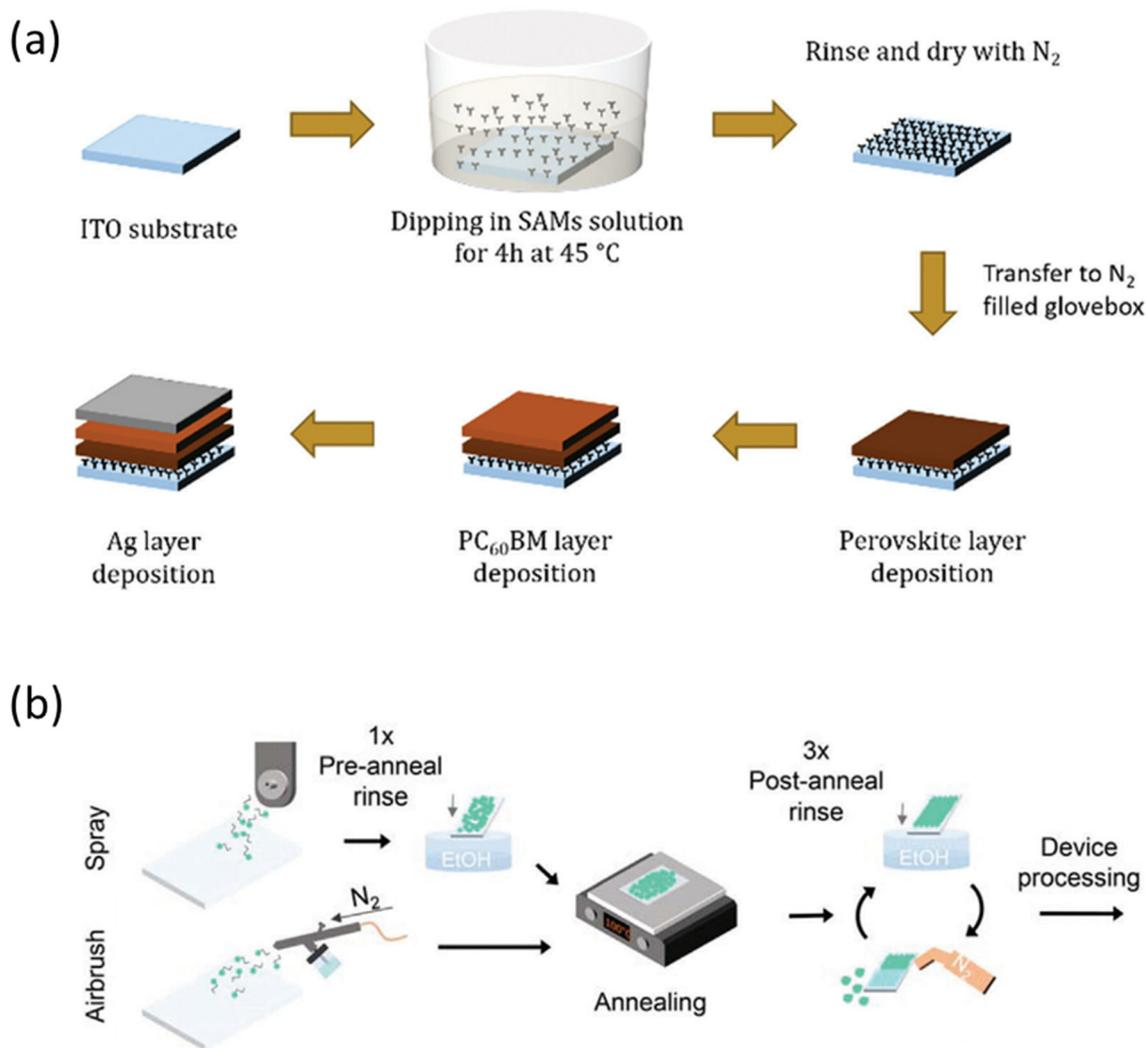
Fig. 2 (a) The dipping process to deposit SAMs onto ITO substrate. Reproduced with permission.<sup>29</sup> Copyright 2019, RSC. (b) The processes of spray- and airbrush-coated SAMs. Reproduced with permission.<sup>30</sup> Copyright 2022, Wiley.
