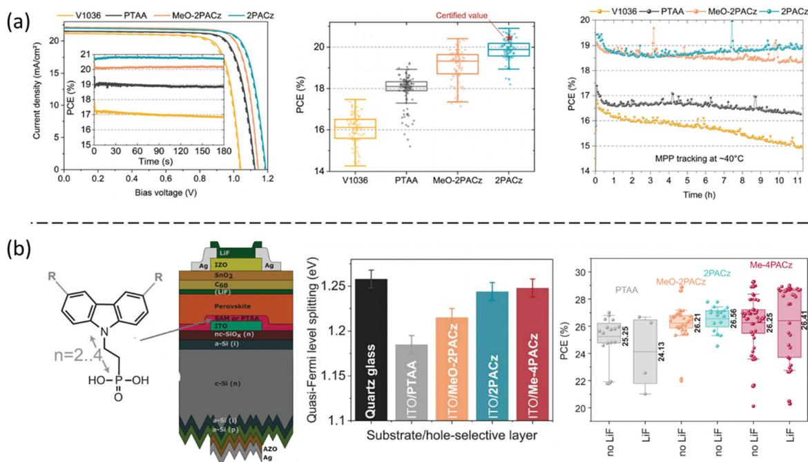
Fig. 6 (a) The device performance of carbazole-based SAMs with phosphonic acid anchoring group. Reproduced with permission.<sup>19</sup> Copyright 2019, RSC. (b) Structure of the perovskite/silicon tandem cell made with SAMs as hole selective contacts. Reproduced with permission.<sup>26</sup> Copyright 2020, AAAS.
