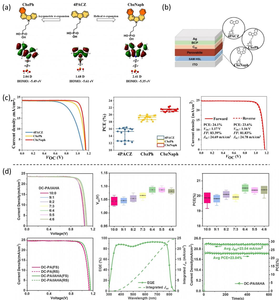
Fig. 7 (a) The  $\pi$ -expanded carbazole-based molecules and their calculated molecular dipole. (b) Device architecture of the CbzPh and CbzNaph-based p-i-n PSC and (c) their corresponding device performance. Reproduced with permission.<sup>27</sup> Copyright 2022, Wiley. (d) Device performance is based on the co-assembled DC-PA and IAHA monolayer substrates. Reproduced with permission.<sup>38</sup> Copyright 2022, Wiley.
