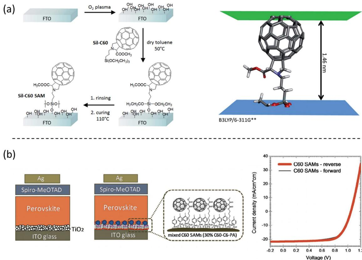
Fig. 11 (a) Illustration of the siloxane-functionalized fullerene self-assembled monolayer fabrication process, and the calculated molecule length. Reproduced with permission.<sup>53</sup> Copyright 2017, RSC. (b) Device structure with fullerene-based SAM electron selective contact and corresponding device performance. Reproduced with permission.<sup>54</sup> Copyright 2017, Wiley.
