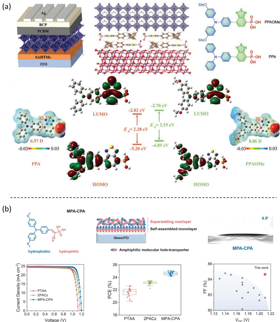
Fig. 8 (a) The molecular structures of PPA and PPAOMe and the corresponding calculated HOMO/LUMO levels. Reproduced with permission.<sup>41</sup> Copyright 2023, Wiley. (b) Schematic depiction of the bilayer stack of MPA-CPA molecules on an ITO-glass substrate and the corresponding device performance. Reproduced with permission.<sup>15</sup> Copyright 2023, AAAS.
