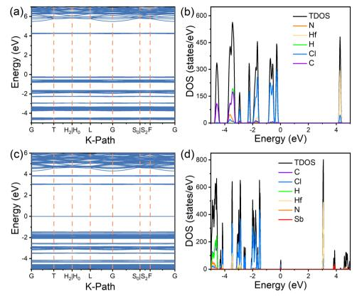
Fig. 4 DFT simulations. (a) electronic band structures and (b) density of states (DOS) of (TMA)<sub>2</sub>HfCl<sub>6</sub>; (c) electronic band structures and (d) DOS of Sb<sup>3+</sup>doped (TMA)<sub>2</sub>HfCl<sub>6</sub>.
