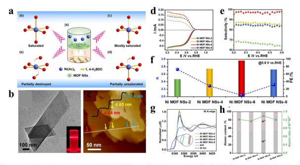
Fig. 2 (a) Illustration of the synthetic method for Ni MOF NSs. (b) TEM and (c) AFM images of Ni-MOF NS-6. (d) LSV curves and (e) H<sub>2</sub>O<sub>2</sub> selectivity. (f) The number of electrons transferred (n) and the Faraday efficiency. (g) XANES spectra for Ni MOF NS-2, 4, 6, 8, NiO and Ni foil. (h) The atomic content of  $Ni^{2+}$ and  $Ni^{3+}$ , and the atomic ratio of  $Ni^{2+}/Ni^{3+}$  in Ni MOF NS-2, 4, 6 and 8. Copyright 2021, WILEY-VCH.
