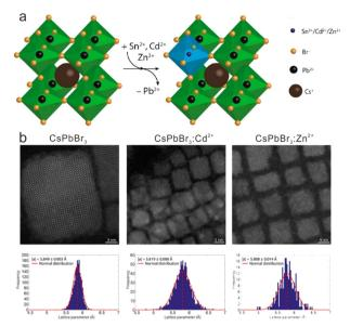
Fig. 5 (a) Schematic illustration of partial cation exchange of host Pb<sup>2+</sup> with guest  $M^{2+}$  ions (M = Mn, Zn and Cd) in CsPbBr<sub>3</sub> NCs. (b) Quantitative high-angle annular dark-field STEM images of CsPbBr<sub>3</sub>, CsPbBr<sub>3</sub>:Cd<sup>2+</sup> and CsPbBr<sub>3</sub>:Zn<sup>2+</sup>. Reproduced with permission from ref. 99. Copyright 2017, American Chemical Society.
