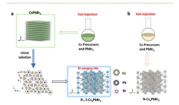
Fig. 1 (a) Schematic of the phase transformation from 3D cubic CsPbBr<sub>3</sub> to hexagonal 0D R- and S-Cs<sub>4</sub>PbBr<sub>6</sub> NCs. (b) Schematic of the synthesis of N-Cs<sub>4</sub>PbBr<sub>6</sub> NCs.
