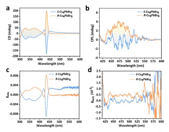
Fig. 3 Chiral characterization of R- and S-Cs<sub>4</sub>PbBr<sub>6</sub> NCs. (a) CD spectra and (c) the corresponding dissymmetry factor g<sub>abs</sub>. (b) CPL spectra and (d) glum of R- and S-Cs<sub>4</sub>PbBr<sub>6</sub> NCs.
