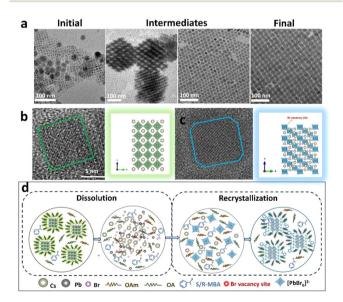
Fig. 4 Transient phases in the conversion of CsPbBr<sub>3</sub> to Cs<sub>4</sub>PbBr<sub>6</sub>: (a) TEM images of the initial Br perovskite NCs and of intermediates upon conversion to the final Cs<sub>4</sub>PbBr<sub>6</sub> product. TEM images and atomic model (b) of cubic CsPbBr<sub>3</sub> (c) and of rhombohedral Cs<sub>4</sub>PbBr<sub>6</sub>NCs. (d) Schematic of the proposed dissolution-recrystallization transformation mechanism.
