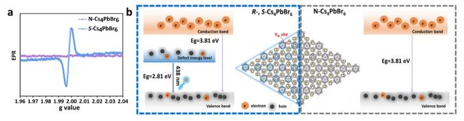
Fig. 5 (a) EPR spectra of S-Cs<sub>4</sub>PbBr<sub>6</sub> NCs and N-Cs<sub>4</sub>PbBr<sub>6</sub> NCs. (b) Schematic of the comparison of electronic band structure and luminescence mechanism for chiral Cs<sub>4</sub>PbBr<sub>6</sub> NCs (left) and N-Cs<sub>4</sub>PbBr<sub>6</sub> NCs (right).
