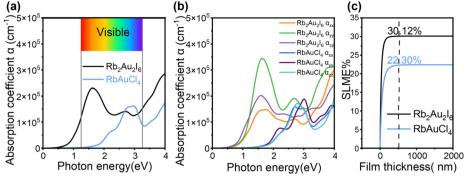
Fig. 4 Optical properties of Rb<sub>2</sub>Au<sub>2</sub>I<sub>6</sub> and RbAuCl<sub>4</sub>. (a) Calculated absorption spectra of average optical directions and (b) different optical polarizations. (c) SLME as a function of film thickness.
