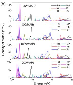
Fig. 5 DOS of the relaxed perovskite/BaWO<sub>4</sub> interfaces: (a) CsPbBr<sub>3</sub>/ BaWO<sub>4</sub> and (b) MAPbBr<sub>3</sub>/BaWO<sub>4</sub>.
