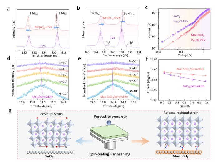
Fig. 4 XPS spectra of (a) Pb 4f and (b) I 3d for the perovskite and Mn(Ac)<sub>2</sub> + perovskite. (c) Dark I-V curves based on SnO<sub>2</sub> and Mac-SnO<sub>2</sub>. Depthdependent GIXRD patterns of the (d) SnO<sub>2</sub>/perovskite and (e) Mac-SnO<sub>2</sub>/perovskite, and their (f) linear fits of  $2\theta - \sin^2 \Psi$ . (g) Residual stress diagram of the SnO<sub>2</sub>/perovskite and Mac-SnO<sub>2</sub>/perovskite.
