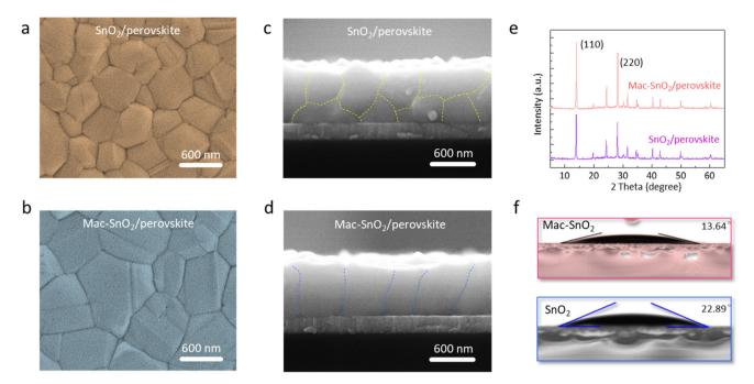
Fig. 3 Top-view and cross-section SEM images of perovskite layers grown on (a and c) SnO2 and (b and d) Mac-SnO2 ETL. (e) XRD patterns of the SnO<sub>2</sub>/perovskite and Mac-SnO<sub>2</sub>/perovskite. (f) The water contact angles on SnO<sub>2</sub> and Mac-SnO<sub>2</sub> films.
