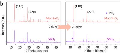
Fig. 7 (a) Normalized PCEs of SnO<sub>2</sub> and Mac-SnO<sub>2</sub> PSCs placed in the ambient environment (25–30 °C, 30%–40% humidity). (b) XRD spectra of the  $SnO_2$ /perovskite and Mac- $SnO_2$ /perovskite before and after exposure to an air environment with 30%-40% humidity for 20 days.
